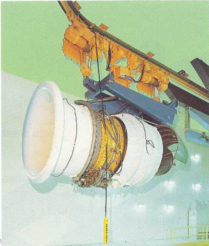
Louden monorail transports jet engine and spring beam into a test cell at an airline maintenance center, for automatic connection of wiring and plumbing.
