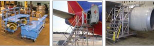
Adjustable Custom Access Solutions provide the ability to operate at a wide range of platform heights. This type of adjustment gives the worker access to various working positions and allows one ladder to replace multiple static height ladders. The adjustment is provided by either hydraulic hand pump or via standard shop air for ease of use.
