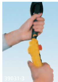
Fit the plug with its bayonet connector into the control pendant and turn until it locks
