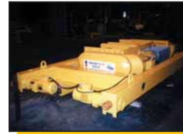
25 ton trolley hoist with flux vector drive In a steel service center
