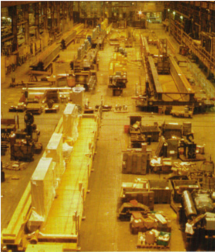
One of the assembly floors where Whiting cranes from 5 to 800 ton capacity receive final assembly and testing.
