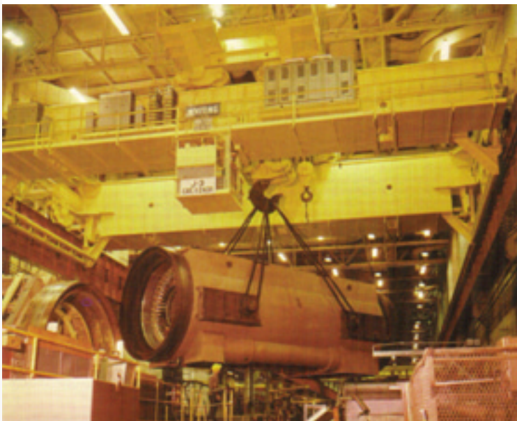
A Whiting 400/50 ton crane used for manufacturing Power plant turbines.
