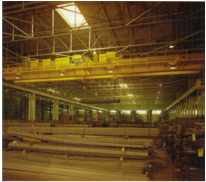
This 25 ton cab operated crane efficiently handles long loads.
